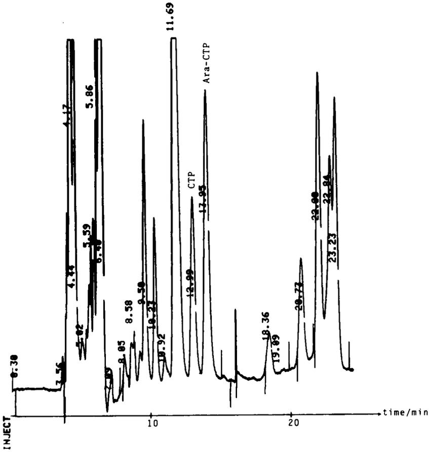
Fig. 3. HPLC separation of eluent-soluble material extracted from the equivalent of  $5 \cdot 10^6$  K562 cells incubated with Ara-C (0.01 a.u.f.s.).
