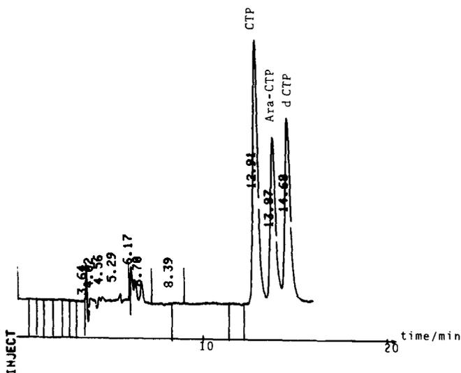
Fig. 1. HPLC separation of a standard mixture of CTP, Ara-CTP and dCTP (10- $\mu\text{l}$  injection, 10  $\mu\text{g}/\text{ml}$  Ara-CTP, 0.02 a.u.f.s.).
