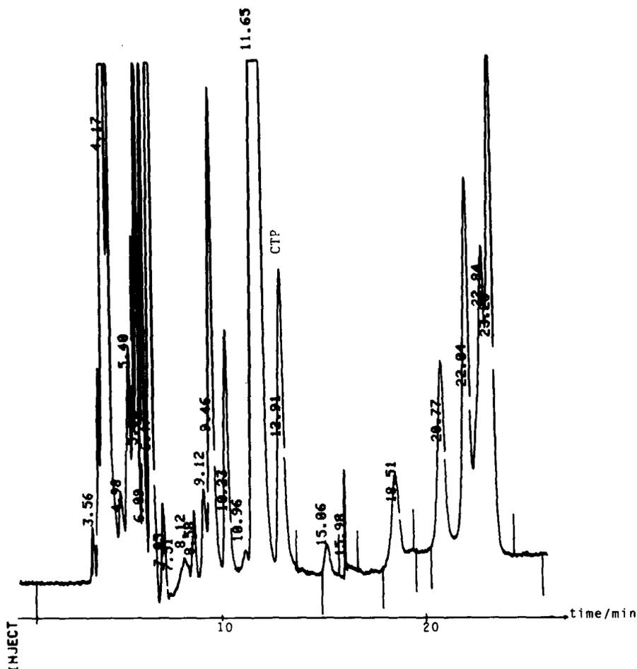
Fig. 2. HPLC separation of eluent-soluble material extracted from the equivalent of  $5 \cdot 10^6$  K562 cells (0.01 a.u.f.s.).
